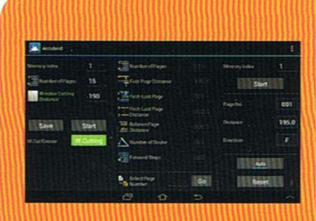
Digital Micro Controller, with a large LCD Touch Screen to pre-define and save each project
